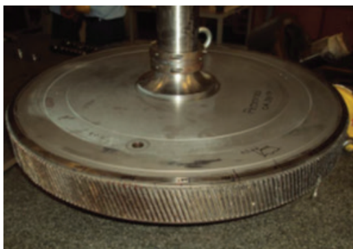
Damaged Input Geat Wheel
